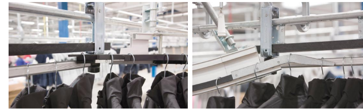
Loading and unloading. Linking of the Slide Rail system to the Trolley system is the most cost effective way of bridging long distances to the static stock.
